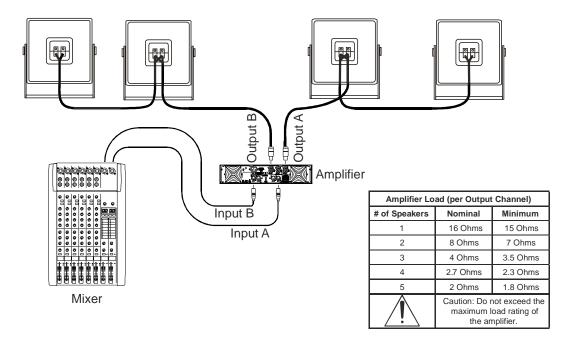
Usually PULCE is used with PULCEW subwoofer (out for PULCE with crossover network at 180Hz 6dB/oct), an example of recommended configuration (PULCEW in stereo mode, 2 PULCE per out) using multiple speakers is represented below:
